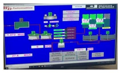
The city of Mount Carmel's waste water treatment facility is a biological processing treatment plant that utilizes grit removal, primary settling and biological treatment to remove residential and commercial sanitary sewage.
